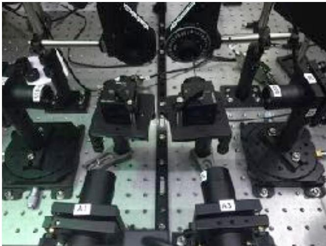
Figure 4 Two PBSs (center),  $\frac{1}{4}$  wave plate (left), Liquid crystal wave plate (right) and fiber couplers (fiber-coupled
